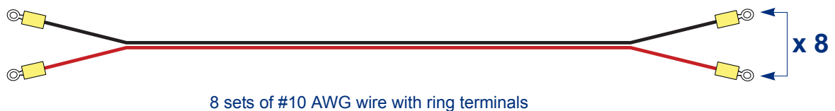
Figure 23. #10 AWG wire for circuit breaker
