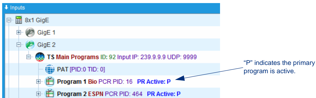
Figure 171. Program Redundancy Indicator — Primary Programs Active
