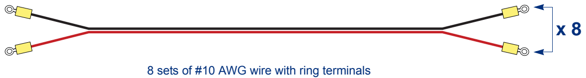
Figure 4. #10 AWG wire for circuit breaker
